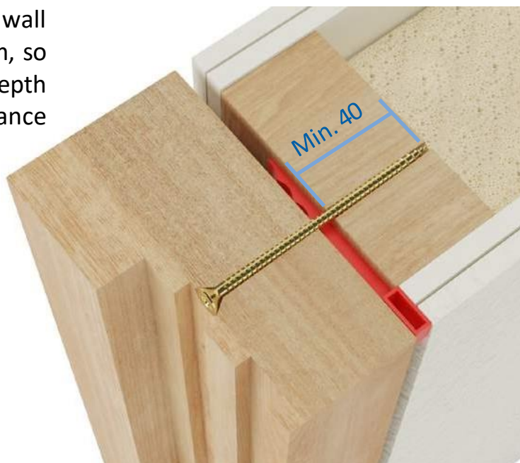
Frame to opening fixings being fitted through the packer
