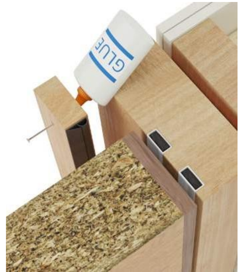
Plant on stop has seals and adhesive applied, and is mechanically fixed to the frame
