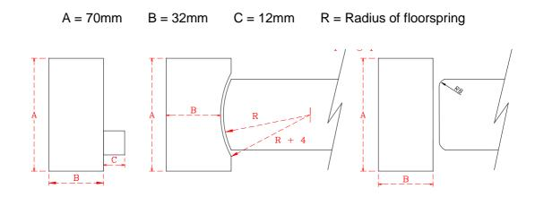
Frame joints may be mortice and tenon, half lapped or mitred, except transoms that must be mortice housed and glued. Frames must be contained within and not offset in relation to the structural opening and must not be rebated adjacent to the door junction. The following diagram depicts acceptable specifications.
