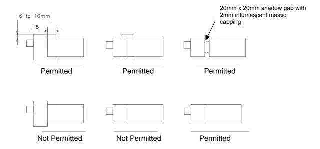
Door frame material may be hardwood with a minimum density of 640kg/m³ and to class J10 as specified in BS EN 942: 1996.
